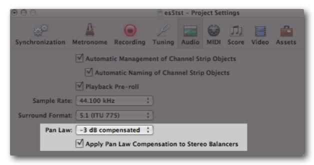
If 'Apply...' is on, Silent Way needs to know about these settings so it can adjust its output
