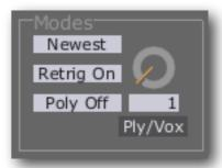
The master plug-in should have its 'Poly Mode' menu set to 'Master'. The adjacent 'Ply/Vox' (short for 'Polyphony/Voice') knob controls the maximum polyphony i.e. the number of simultaneous voices that will sound. This should be set to the number of additional Voice Controller plug-ins that you're going to set up.
