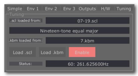
The plug-in requires both a scale definition (.scl) file and a keyboard mapping (.kbm) file. Pressing "Load .scl" allows you to choose the .scl file; similarly "Load .kbm" chooses the .kbm file.
