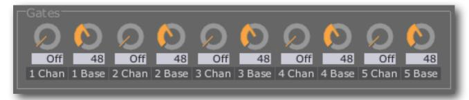
There is a pair of controls for each of the ES-4's 5 channels i.e. the 5 possible Gate Expanders. "Channel" sets the MIDI channel to respond to, or "Off". "Base" sets the base note to respond to, which will control the Gate Expander's output 1. The remaining 7 outputs will be controlled by the 7 MIDI notes above the base note e.g. if the base note is 48, outputs 1 to 8 on the Gate Expander will be controlled by notes 48 to 55.
