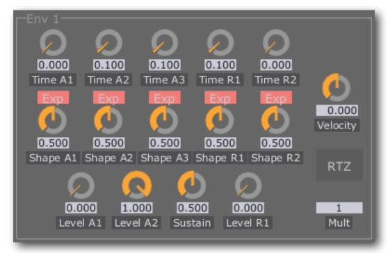
The envelope controls are exactly the same as those of the Voice Controller's envelopes, though the full controls are always displayed. In terms of the Voice Controller's 'simple controls':
