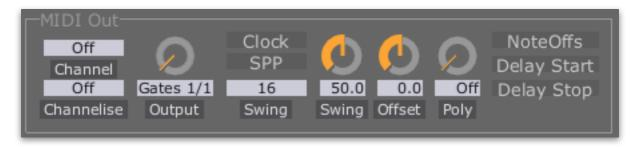
This section allows a Gate Expander output to be used as a MIDI output. Because the ES-4's outputs are derived from an audio signal, the MIDI messages sent from an ES-4 are free from the <u>timing problems</u> often associated with regular (e.g. USB) MIDI interfaces.
