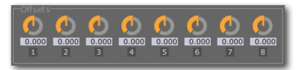
The "Offsets" controls let you dial in a voltage offset on each ESX-8CV output. The values on the controls are in Volts (assuming the ESX-8CV's jumper is not fitted, and the calibration trimmer is at the factory default setting).
