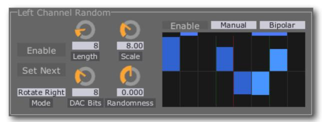
Pressing the 'Random' button shows controls for the Step LFO's random step generator.
