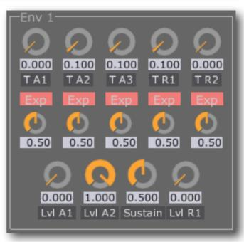
The 'Exp' button toggles the curve type between parabolic and exponential.
