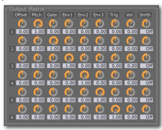
The Output Matrix section lets you select which of the plug-in's output signals appear on which of the six plug-in outputs.
