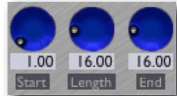
The Start knob always sets the start position of the pattern; the end of the pattern is set by the Length knob if the Length Mode menu is set to 'Start/Length' and by the End knob if the Length Mode menu is set to 'Start/End'.
