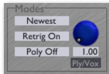
'Master'. The adjacent 'Ply/Vox' (short for 'Polyphony/Voice') knob controls the maximum polyphony i.e. the number of simultaneous voices that will sound. This should be set to the number of additional Voice Controller plug-ins that you're going to set up.
