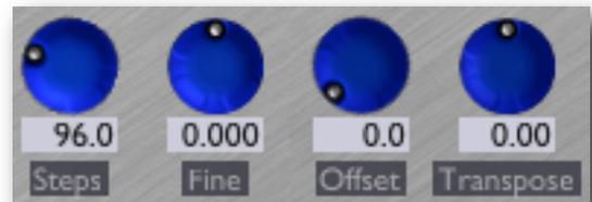
The 'Offset' control sets where within a step the zero line sits - refer to the video as mentioned above for clarification.
