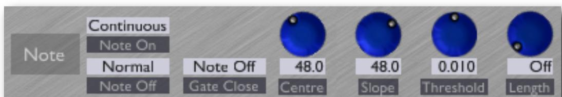
Both note on and note off messages can be generated. The three drop-down menus select the behaviour of the plug-in in terms of when messages are sent.
