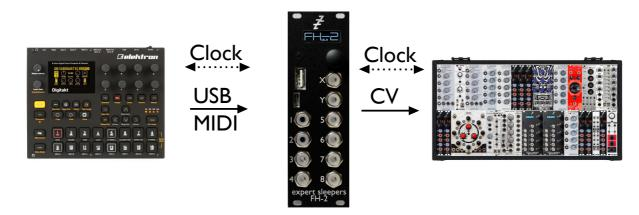
Multiple clock outs at different divisions, run/stop triggers etc. Groovebox, FH-2, or another module can be the clock master.
