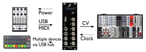
Up to 64 outputs. Direct control of CVs from faders, flexible and syncable LFOs, triggers from pads etc.
