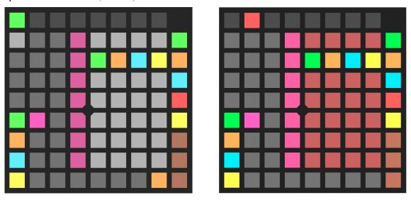
The 4x7 grid of white (load) or red (save) buttons represent the 28 sequence slots. The slots most recently accessed by the four sequencers are indicated with green, orange, blue or yellow highlights
