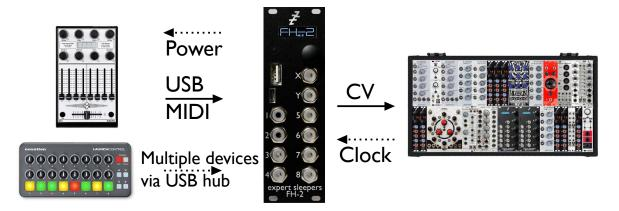
Up to 64 outputs. Direct control of CVs from faders, flexible and syncable LFOs, triggers from pads etc.
