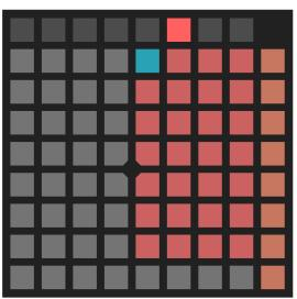
The 4x7 grid of white (load) or red (save) buttons represent the 28 sequence slots. The slot most recently accessed by the drum sequencer is indicated with a blue highlight. Pressing the button for a sequence slot loads or saves the drum sequencer's sequence from or to that slot.
