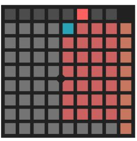
The 4x7 grid of white (load) or red (save) buttons represent the 28 sequence slots. The slot most recently accessed by the drum sequencer is indicated with a blue highlight. Pressing the button for a sequence slot loads or saves the drum sequencer's sequence from or to that slot.
