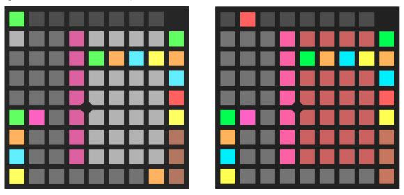
The 4x7 grid of white (load) or red (save) buttons represent the 28 sequence slots. The slots most recently accessed by the four sequencers are indicated with green, orange, blue or yellow highlights
