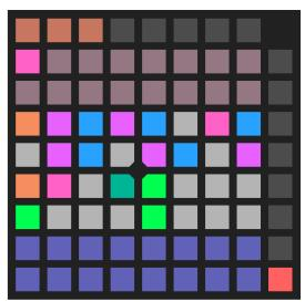
Rows 7 & 8 indicate the current Euclidean pattern being controlled (1 is top left, 16 is bottom right). Press one of these buttons to switch the current pattern.
