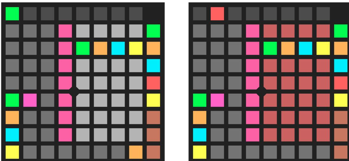
The 4x7 grid of white (load) or red (save) buttons represent the 28 sequence slots. The slots most
