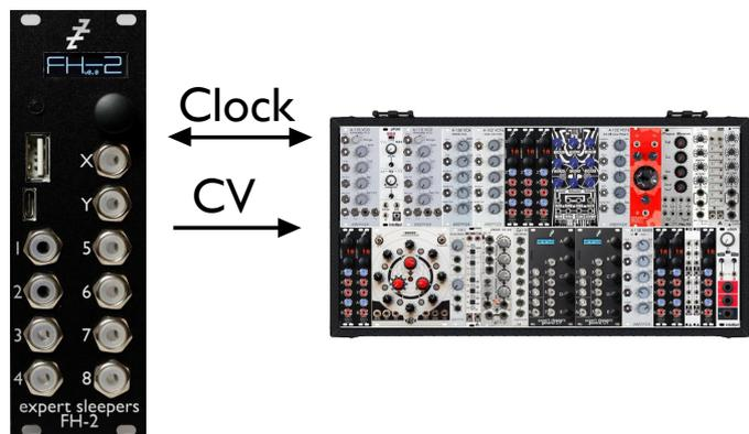
The FH-2 can operate as the clocking centre of your modular, also generating (syncable) LFOs, with no USB connection.
