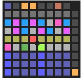
Rows 1-4 show all 32 steps of the lane. The current step is highlighted magenta. Steps within the start and end points are shown white (off) or green (on). As in the overview, pressing a button for a step toggles it on or off, and accents are set by holding button 7/9 and pressing the step button. Note that you can edit steps that are not within the start & end points (shown blue).
