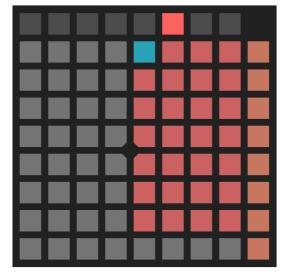
The 4x7 grid of white (load) or red (save) buttons represent the 28 sequence slots. The slot most recently accessed by the drum sequencer is indicated with a blue highlight. Pressing the button for a sequence slot loads or saves the drum sequencer's sequence from or to that slot.
