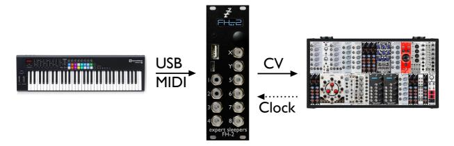
Up to 16 note polyphonic conversion, with optional pitch/gate/velocity etc. CVs per note. Also features arpeggiation, keyboard splits and more.
