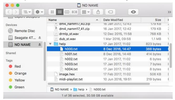
i.e. the 'help' folder is at the root level of the card, and inside is a file per algorithm, named 'hXXX.txt', where XXX is the algorithm number, starting from zero for algorithm A1.
