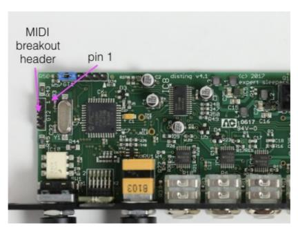
All of the necessary electronics are on the PCB; all that needs to be added is the actual sockets. The header pin-out is as follows:
