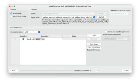
You can then click on the "Start" button (bottom left) to actually perform the firmware update. This should take maybe 15 seconds, and show "Success" when done. Turn the module off and back on to resume normal operation. You may like to check that the "About" screen shows the expected firmware version.
