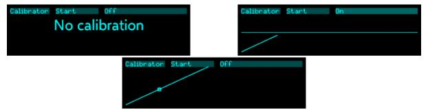
Once the calibration is complete, the algorithm will continuously modify the pitch CV it receives to achieve the expected frequency from the VCO.
