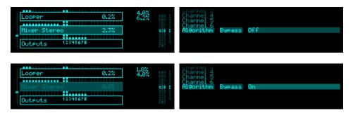
When bypassed, an algorithm appears in the overview 'grayed out'.
