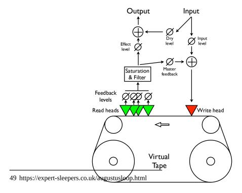
There are four 'tape read heads' with independent delay times and stereo positions, allowing for straight stereo delays, ping pong delays, or hybrid multi-tap style effects.
