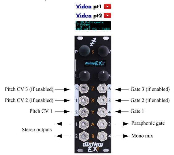
The SD Multisample algorithm is an eight voice polyphonic, three part multitimbral, sample playback instrument, playing WAV files from the MicroSD card. It can have up to 3 input CV/gate pairs, or can be played via MIDI or I2C. It supports both velocity switches and round robins per sample.
