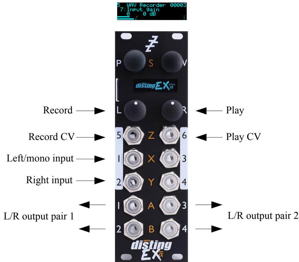
This algorithm records audio (or CV) to the MicroSD card as a WAV file. It can record mono or stereo files at 48 or 96kHz, 16 or 24 bit. It can also play previous recordings, though the various WAV playing algorithms offer many more possibilities.
