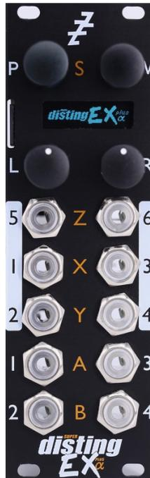
The disting EX has six analogue inputs and four analogue outputs on 3.5mm TS jack sockets. These are designed to cope with any Eurorack signal (with a range of approximately  $\pm 10V$ ), and are DC coupled, so can be used for CVs as well as audio.
