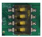
These are used to choose the configuration to load at power on. Please see the section on saving and loading configurations, below.
