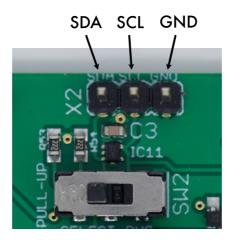
Make or remove I2C connections with the power off.
