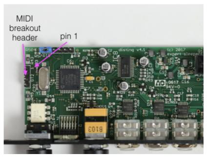
All of the necessary electronics are on the PCB; all that needs to be added is the actual sockets. The header pin-out is as follows:
