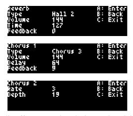
All modes offer two global audio effects, Reverb and Chorus, though both can in fact offer a wider range of effects than the name suggests. The synthesizer voices have independent effects sends to these two effects processes, and indeed the drum parts have per-drum settings for reverb and chorus depth.
