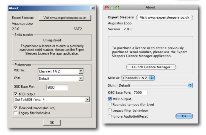
The top section shows the product version. The Windows version also shows which SSE variant has been detected (there are optimised versions of the core processing routines for systems with SSE2).
