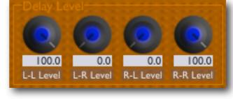
stereo delay. The left-to-right and right-to-left taps allow you create ping-pong style delays. By mixing all four, you can get some spacious stereo spread effects.
